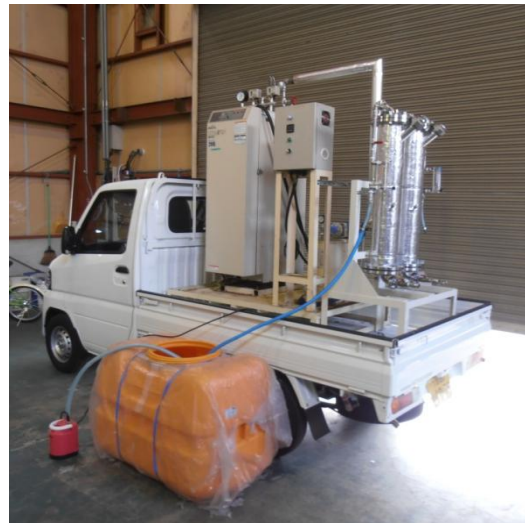
[Small mobile water purification system] (treatment capacity: 5 m 3 /day)
