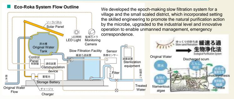
Supply of delicious water is enabled by fully utilizing the natural function of the microbe. Recently this traditional method of the slow filtration trends to be reevaluated in Japan.
