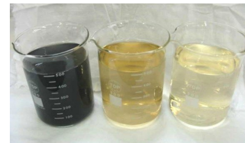
Light: Raw water Middle: After contact oxidation tank Right: After advanced oxidation process
