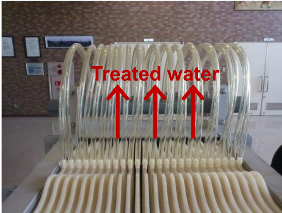
Top of membrane filter unit
