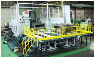
NC Horizontal Boring Machine with Automatic Pallet Changer
