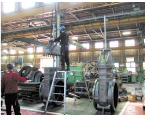
Assembly of Gate Valves
