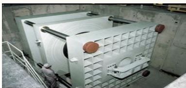
Hydraulic Testing Equipment for Large Size Valves ( 3000φ)
