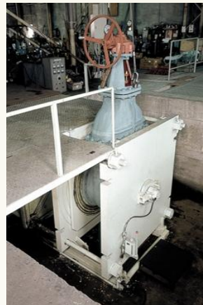
Hydraulic Testing Equipment for Large Size Valves ( 1500φ)
